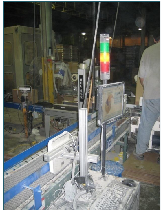
Figure 3: RFID Commissioning Station from Ship2Save
