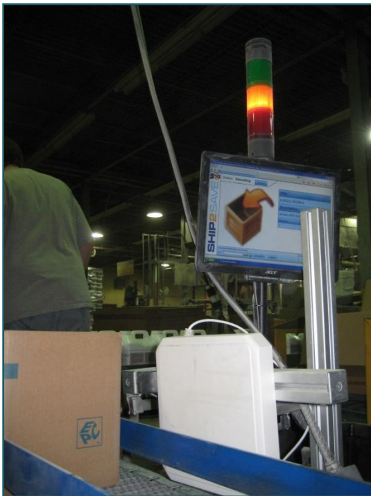
Figure 2: EPC-Ready Case Being Encoded on a Normerica Case Packing Conveyor
