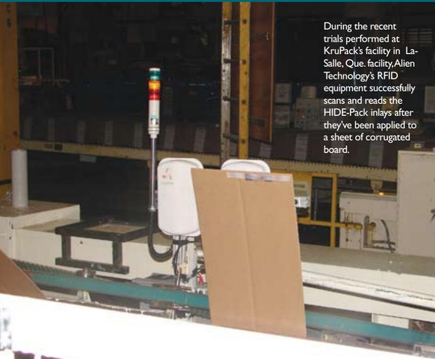
During the recent trials performed at KruPack's facility in LaSalle, Que. facility, Alien Technology's RFID equipment successfully scans and reads the HIDE-Pack inlays after they've been applied to a sheet of corrugated board.
